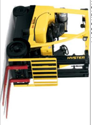
Approved areas of operation... Maximum allowable load on forks <u>1200 lbs</u> ~RCF level 1 Vault lid (Zone E) ~RCF Levels 2-4 ~Level 5 Zone D, E and F All other areas use load chart for max load Allowable loads set by the Structural Engineer
